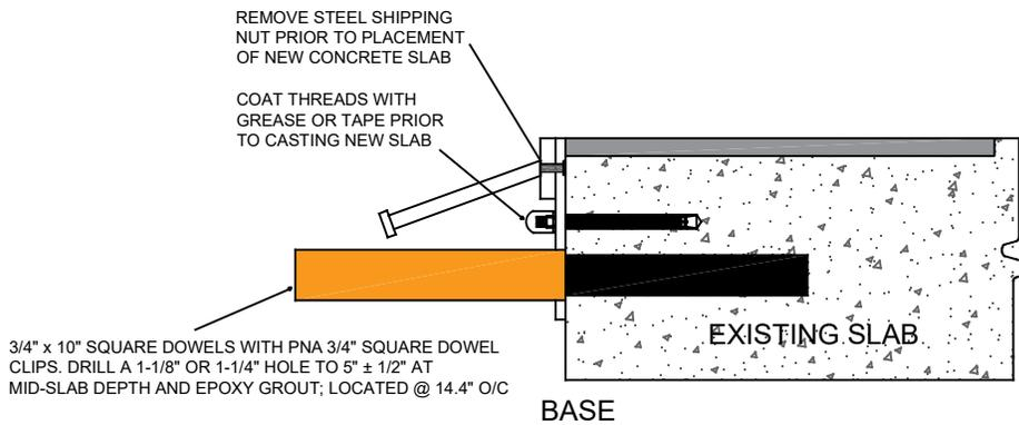
**B** Installation of Square Dowels and Square Dowel Clips
