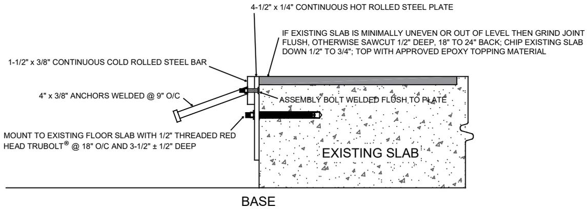
**A** Mount n2e to Existing Slab with Red Head Trubolt®
