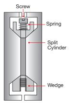
shrinkage or thermal contraction. Installation of each cylinder can be completed in minutes. And because it's a mechanical device that doesn't involve chemical curing like sub-slab injection and retrofit doweling, the floor can be brought back into service immediately after installation.
