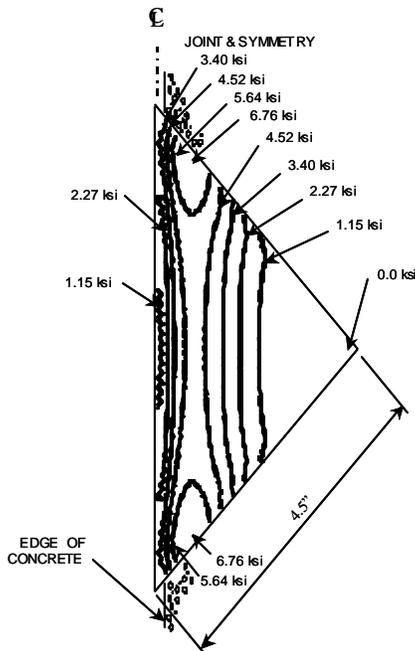
Fig. 3b. FLEXURAL STRESS CONTOURS FOR A 1/4" THICK DIAMOND PLATE DOWEL WITH A ONE KIP LOAD APPLIED TO THE EDGE
