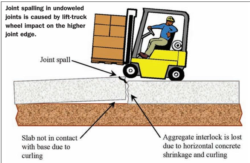
that shows it to be cost effective to use a small portion of these “hidden maintenance costs” to provide dowels in the initial construction to minimize the joint deterioration and equipment repair costs. The payback period for this investment in dowels is as short as 18 months.
