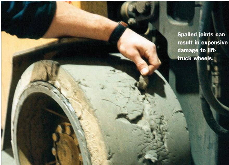
Spalled joints can result in expensive damage to lift-truck wheels.
